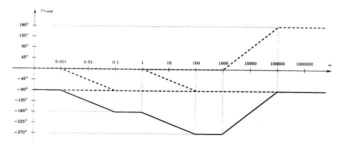
In order to determine the gain and phase margins, we first need to determine the phase and the gain-crossover frequencies.
