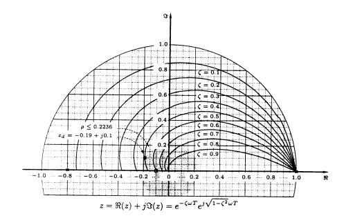
The deficiency angle,  $\phi$ , needed at the desired location to ensure that one of the root-locus branches goes through the location, can be determined from the angular condition.
