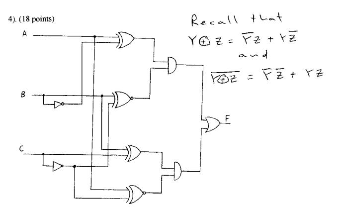
a) Obtain the minimal SOP form for the function "F" using Boolean algebra.
