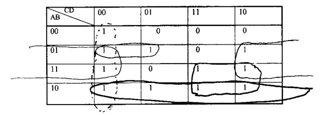
$$F = \overline{CD} + A\overline{B} + AC + \overline{A}B\overline{C} + B\overline{D}$$
