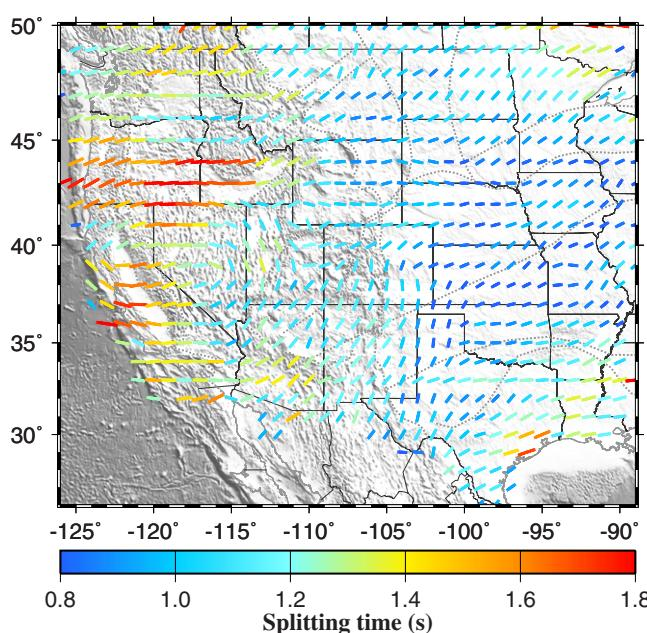
**Figure 5.** Spatially averaged (in radius = 1° circles) shear wave splitting parameters. The color of the bars represents the splitting time.
