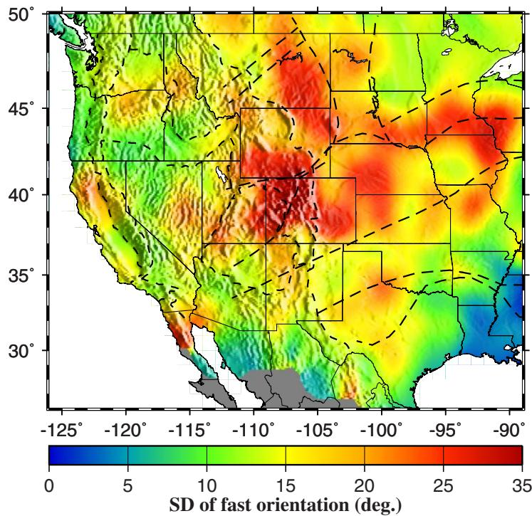
**Figure 12.** Distribution of the standard deviation of spatially averaged fast orientations. The results plotted were resampled into a resolution of  $0.1^\circ$  and spatially smoothed by a cosine arch filter with a radius of  $2^\circ$ .
