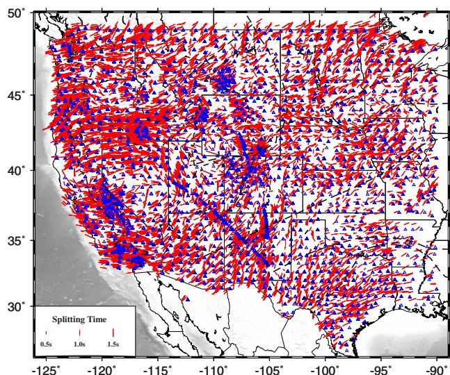
**Figure 2.** Map showing 16,105 pairs of XKS shear wave splitting measurements in the database plotted at the surface projection of the ray-piercing points at the depth of 200 km. Stations are shown as triangles.
