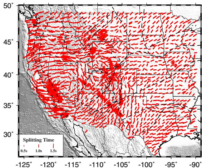
**Figure 4.** Station-averaged shear wave splitting measurements. The averaged fast orientation of a given station was calculated by the circular mean of the individual fast orientations from the station, and the averaged splitting times were produced by averaging the individual splitting times.
