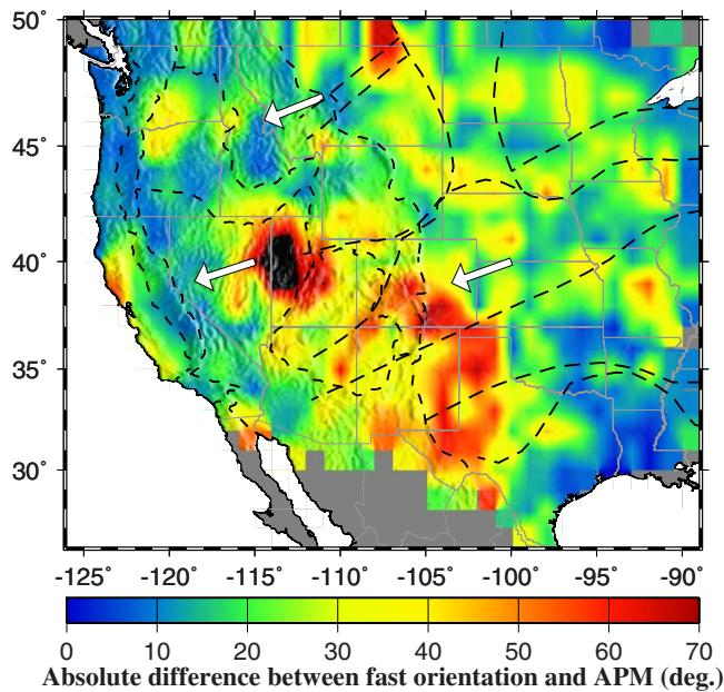
**Figure 6.** Absolution differences between the fast orientations and absolute plate motion (APM) directions of the North American plate determined by the HS3-NUVEL1A model [Gripp and Gordon, 2002]. The white arrows represent the APM directions of the North American plate.
