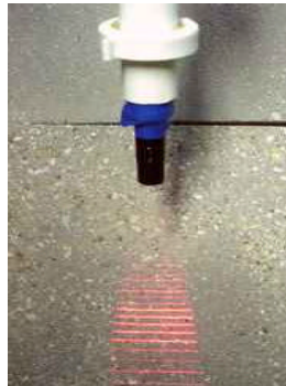
Figure 6, left: CCD camera. Figure 7, center: Line laser. Figure 8, right: Image of a concrete surface being illuminated by an 11-line generator.
