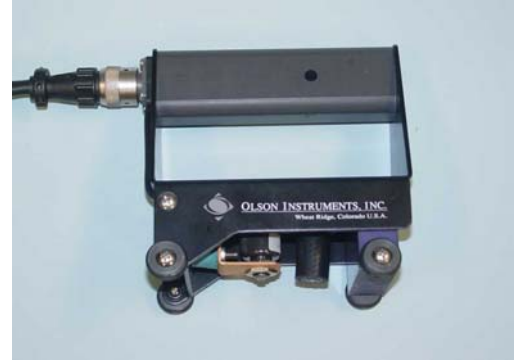
Figure 6: Impact echo tester modified with air coupled receiver.
