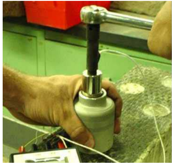
Figure 8: Pull-off tester; destructive testing.
