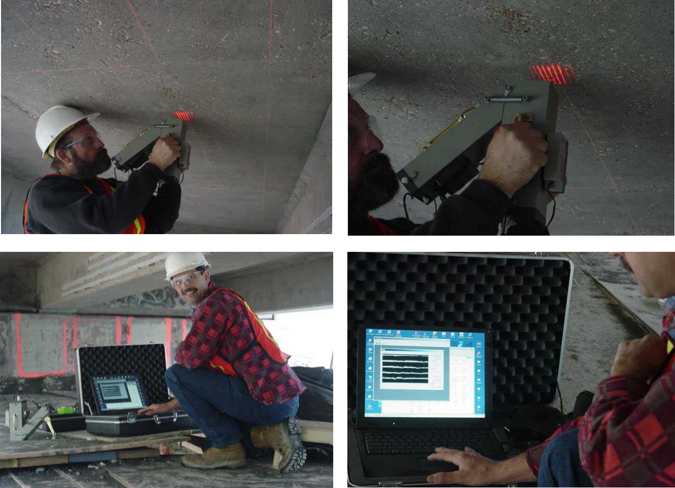
Figure 10: Roughness measurements on the bridge deck.
