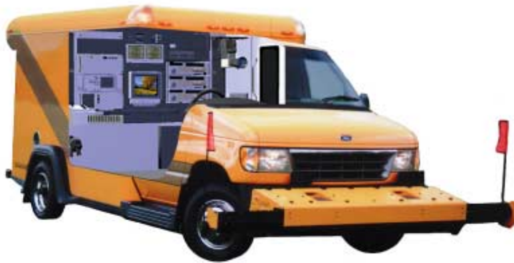
Figure 6. Cutaway of the data acquisition vehicle showing video cameras, computers, video recorders and camera.
