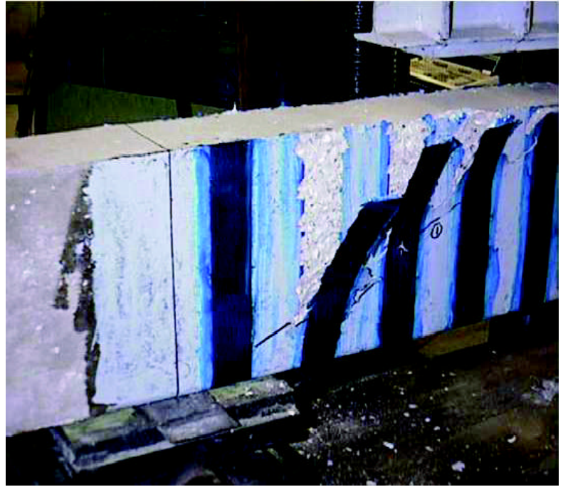
Fig. 2: Delamination of externally bonded FRP sheets
