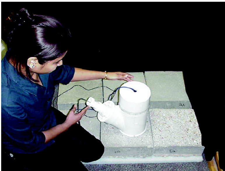
Fig. 5: Prototype of the laser profiling device, measuring six manufactured concrete surface profiles
