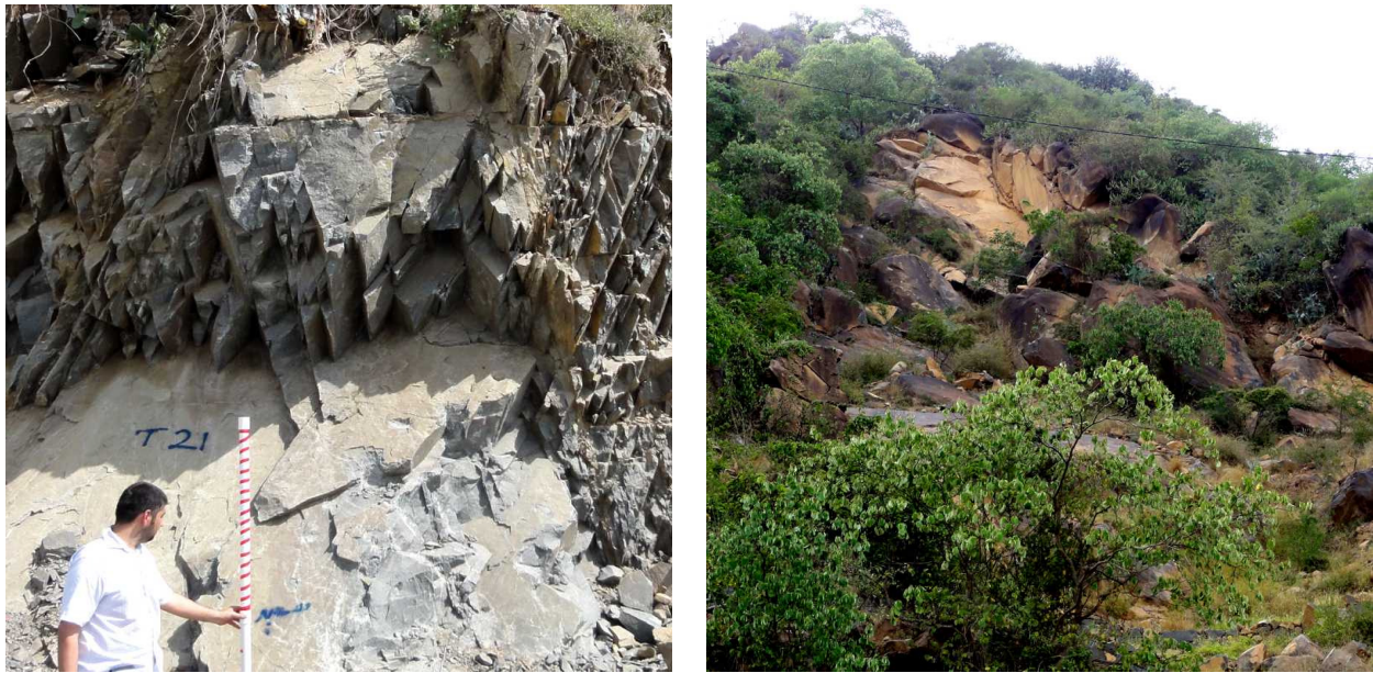
Figure 8: Left: Rock faces with 100% coverage of natural joint surfaces. Right: Rock faces with significant ambiguity as to the location of natural joint surfaces.
