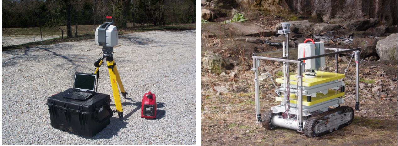
Figure 7: Left: Leica ScanStation II time of flight scanner with integrated optical camera. Right: Leica HDS 6000 phase shift scanner on remote controlled robotic buggy.
