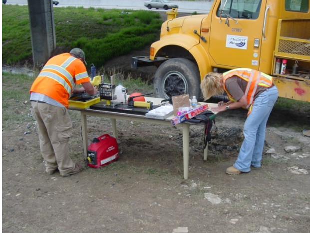
Figure 4. Graduate student Kerry Magner and MoDOT's Sherri Stevens performing point load index tests at test site in Kansas City, Missouri.
