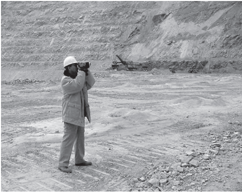
Figure 3. A roving camcorder used to image a muckpile.
