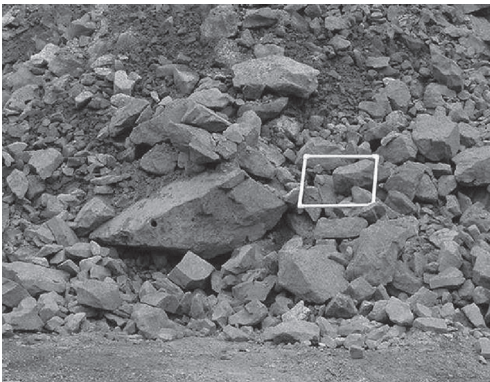
Figure 4. Typical image of a muck pile taken with a roving camcorder; there is a scaling device in the foreground of the image.
