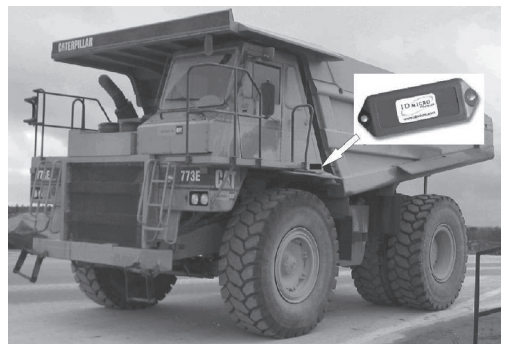
Figure 12. A Haul Dump (HD) truck with an RFID tag.
