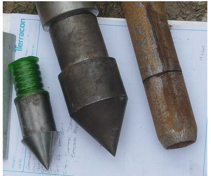
Figure 3: Driven tools. Right: split spoon. Center: Texas Cone. Left: Expendable tip cone.
