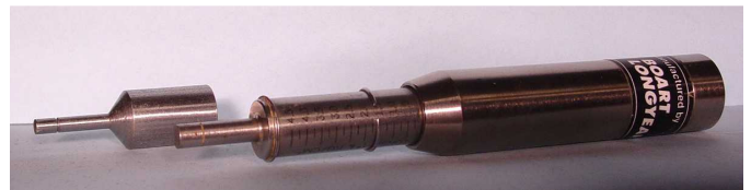
Figure 15: Specially modified pocket penetrometer. With indentation cross section one half of the standard size.
