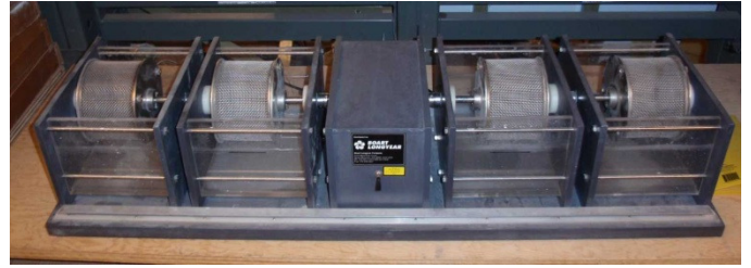
Figure 2: Shale durability testing apparatus.
