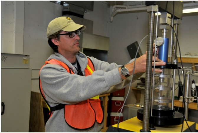
Figure 12: Triaxial testing in MODOT field office. (Photo: Dory Colbert)
