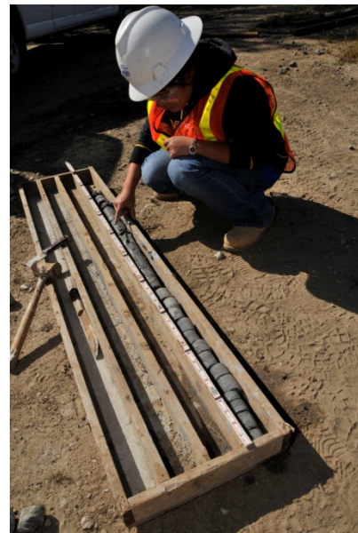
Figure 11. Shale core samples for on-site triaxial strength testing. Samples were wrapped in plastic wrap and foil and transported to an on-site laboratory within five hours of sampling. (Photo: Dory Colbert)
