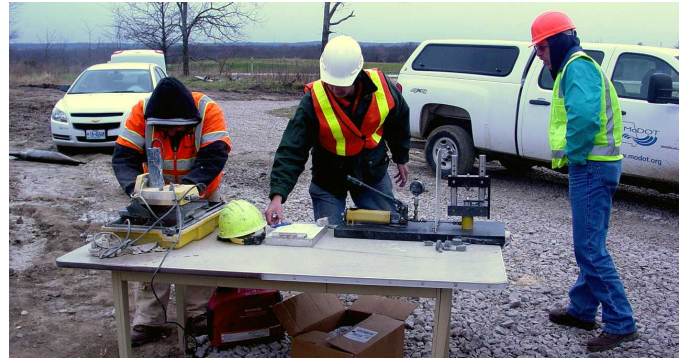
Figure 14: Point load testing in the field. Because axial testing was deemed necessary, a tile saw was used in the field to prepare samples.
