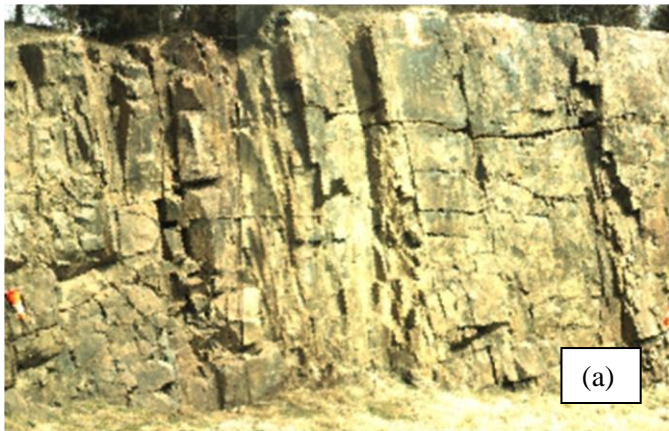
Figure 14: Discontinuity Trace Measurements from the Optical Image. (a) Original optical image; (b) linear trace components detected by canny edge detector; (c) reconciled co-linear trace components by using line fitting. Traces are clustered based on their direction. Six clusters of linear traces, traces of the same cluster are displayed using the same color; (d) directions of the six clusters of the linear traces. Each cluster is shown in one color.
