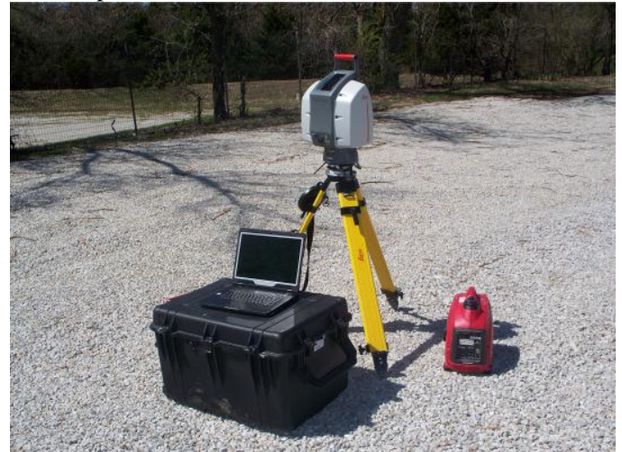
Figure 5: Leica ScanStation 2 LiDAR unit.
