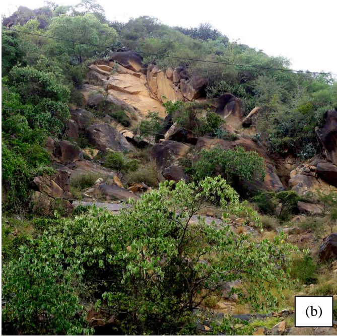
Figure 4: Rock faces with 100% coverage of natural joint surfaces (a) and with significant ambiguity as to the location of natural joint surfaces (b).
