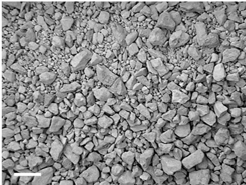
n=2.0. Characterized by a fairly uniform size distribution, where the smallest common visible block is about 1/5 the size of the largest common block. The ratio of the number of largest common blocks to smallest common blocks is about 20:1. (The white scale bar represents 1 inch.)
