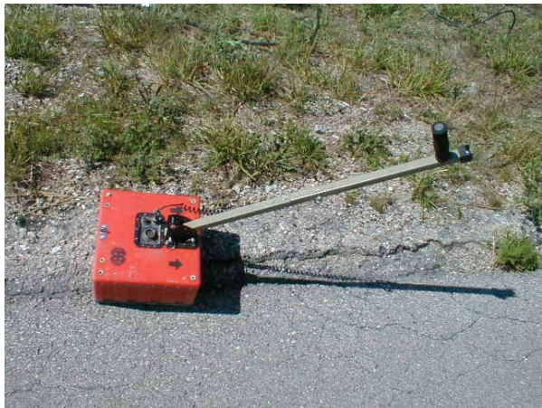
Figure 7. SIR10B ground penetrating radar system, showing a 400 MHz. antenna.
