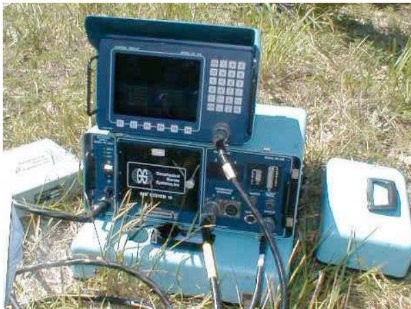
Figure 7. SIR10B ground penetrating radar system, showing a 400 MHz. antenna.
