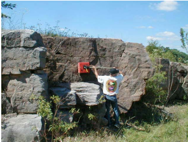
Figure 8. Site 1 with a 2" soil filled vertical joint, 7' deep into the rock.
