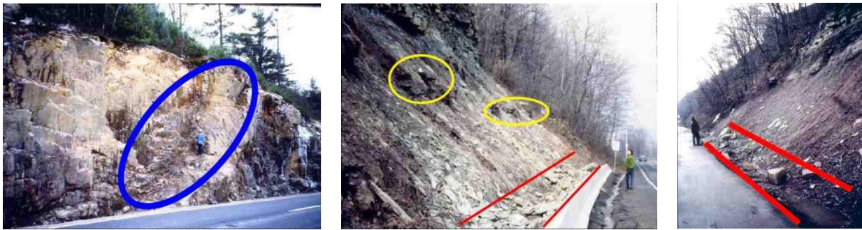
Figure 8. Simulated images demonstrating the potential to develop mobile vision based data acquisition systems for rudimentary measures such as slope heights, slope angles, loose rock quantities and ditch capacities
