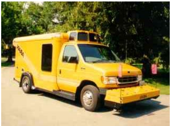
Figure 7. The ARAN system, a mobile instrumented video data collection vehicle designed to take video images at highway speeds and allow users to make measurements and create roadside inventories (Maerz and McKenna, 1999).
