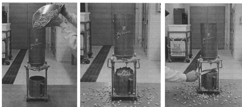
Fig. 2. Uncompacted voids test for measuring void ratio/coarse aggregate angularity
