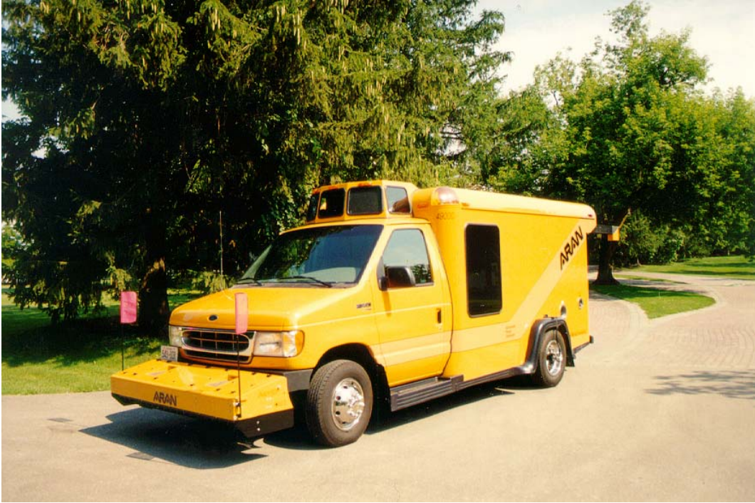
Figure 1. An example of an Automatic Road Analyzer (ARAN) made by RoadWare Corporation.
