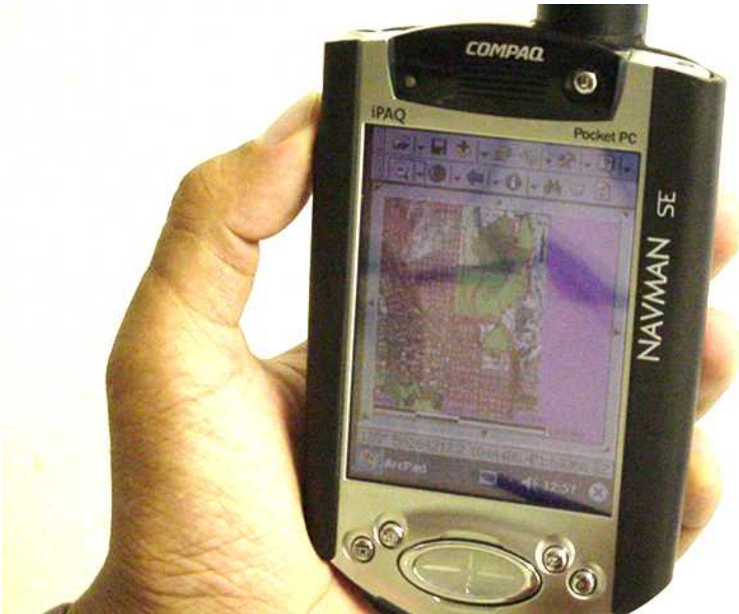
Figure 6. Compaq IPAQ PC with ArcPad software for field data collection.
