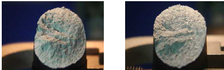
Figure 8: Sample G2 matching surfaces, as an example of the samples used in Table 1 (surfaces created in aluminium using static tensile force).
