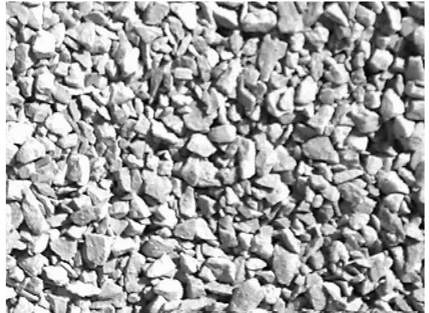
Figure 3: Minus ½” crusher run product from on an aggregate quarry belt
