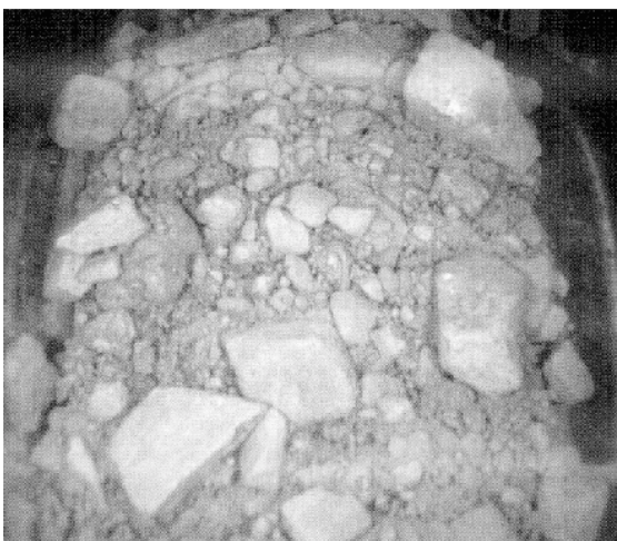
Figure 6. Typical Highland Valley copper image of ore free falling off the end of a transfer chute, and the WipFrag generated block outlines (Simkus and Dance, 1998).
