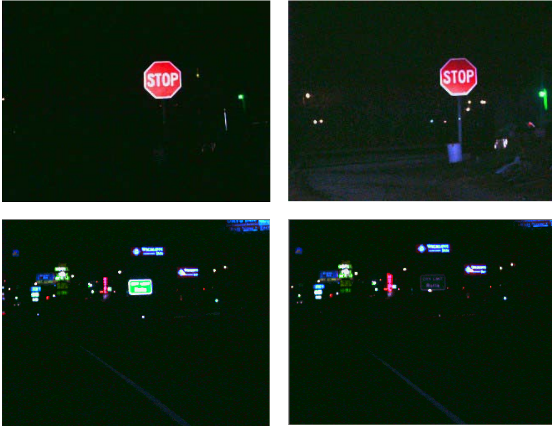
FIGURE 7 Top left: High beam image. Top right: Low beam image. Note increase of background noise. Bottom left: High beam image. Bottom right: Low beam image. Note that the green sign in the left image almost completely disappears in the cluttered background of “lit” signs
