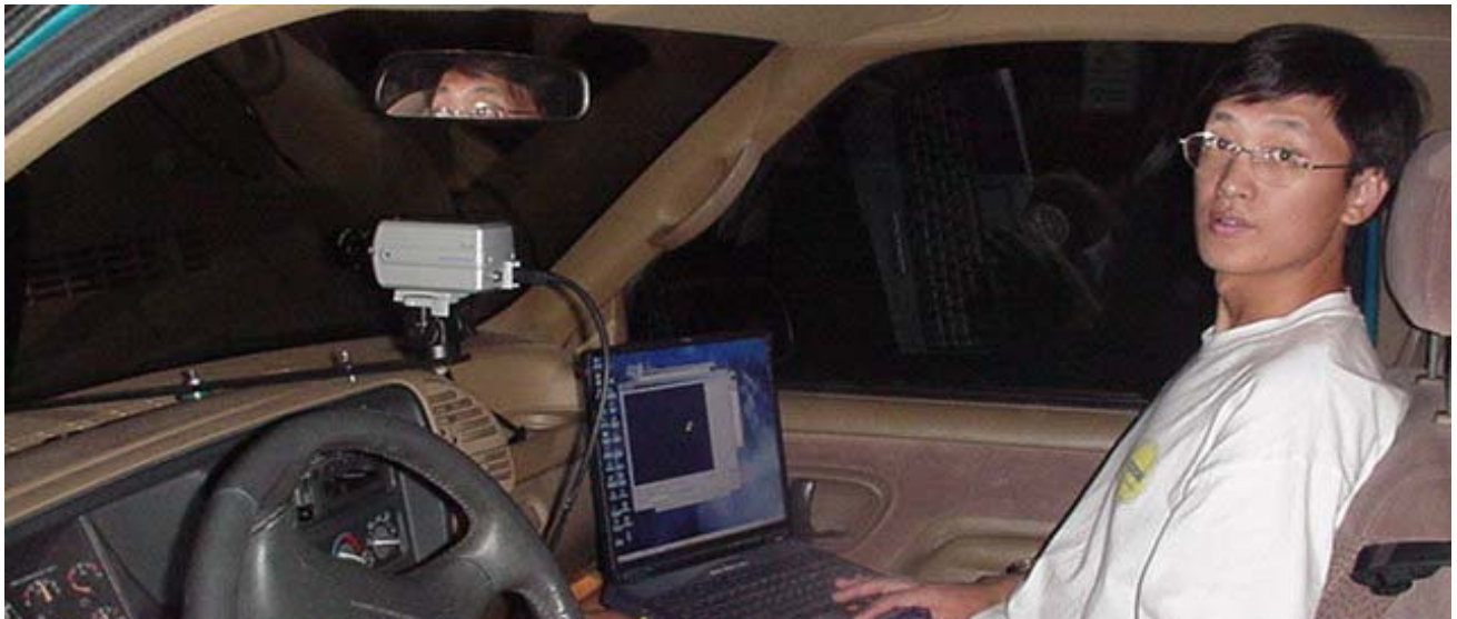
FIGURE 1 Top: Stop sign illuminated by headlights of a vehicle. Bottom: In-vehicle installation consists of a dash mounted digital camera, attached to a laptop computer.
