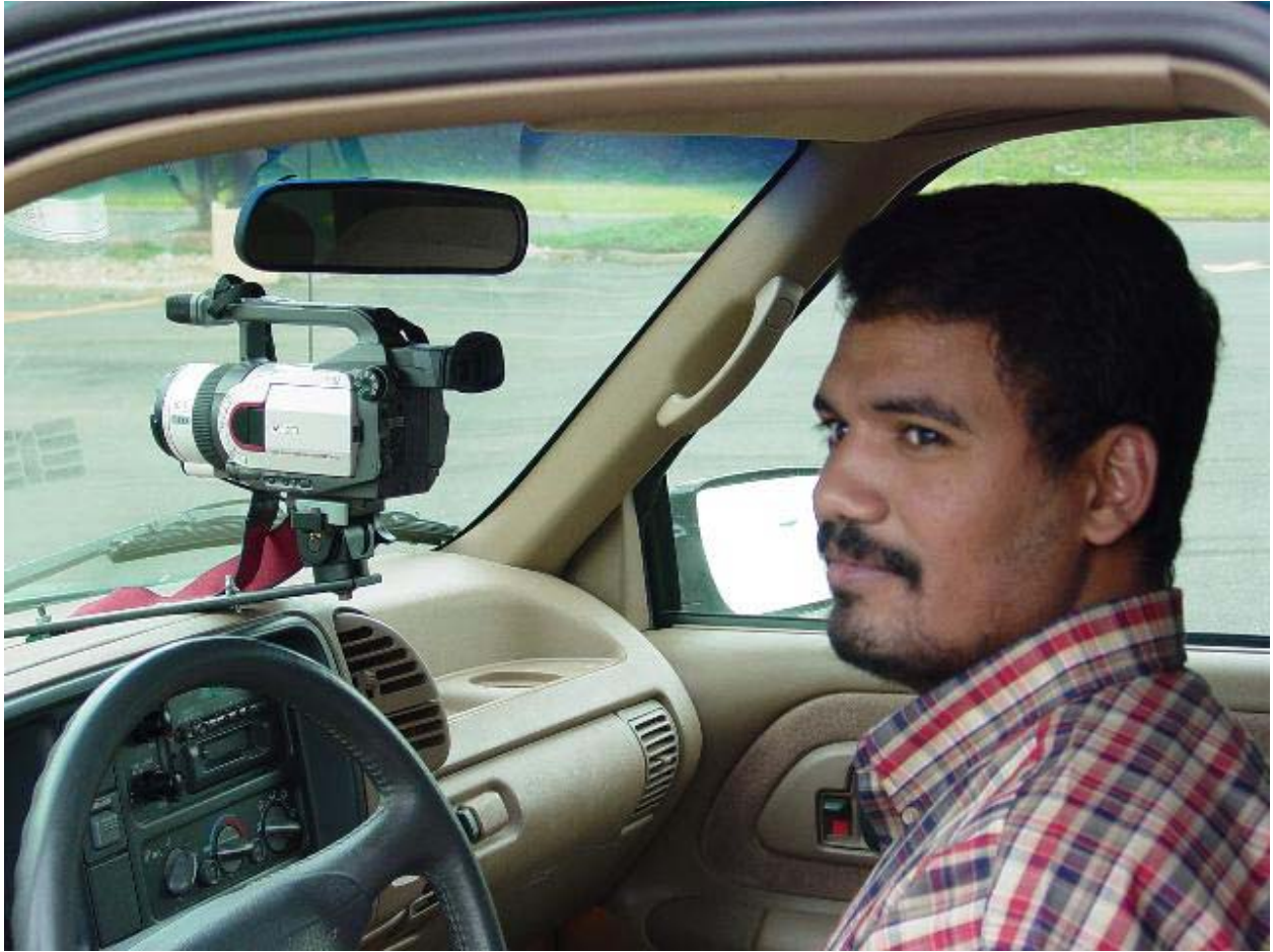
FIGURE 1 Digital camcorder mounted on vehicle dashboard.
