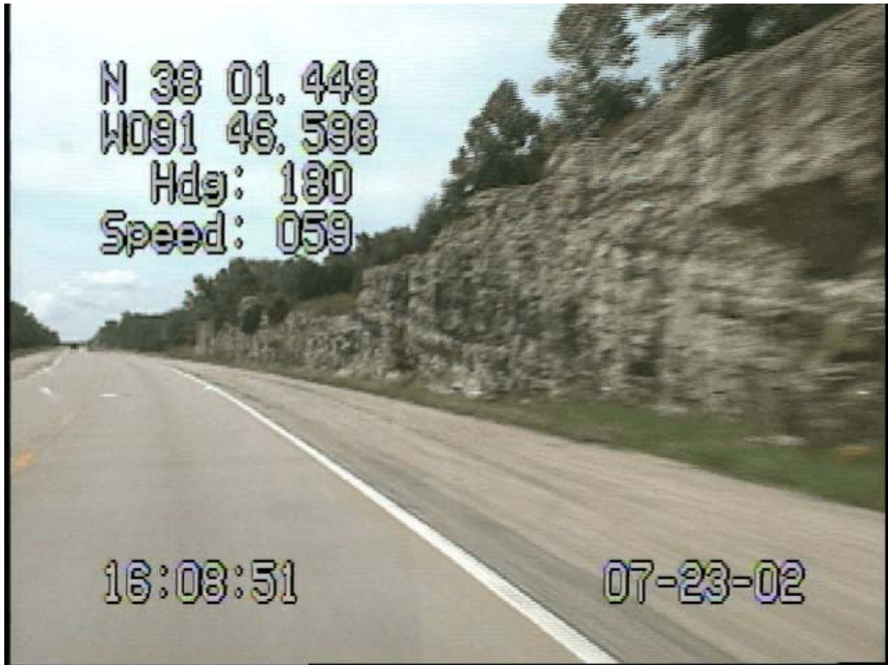
FIGURE 2 Video frame with overlain GPS coordinates, heading, speed, time, and date.
