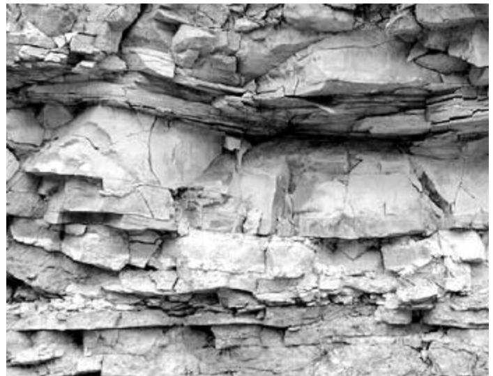
Fig. 1. The discontinuous nature of rock masses.
